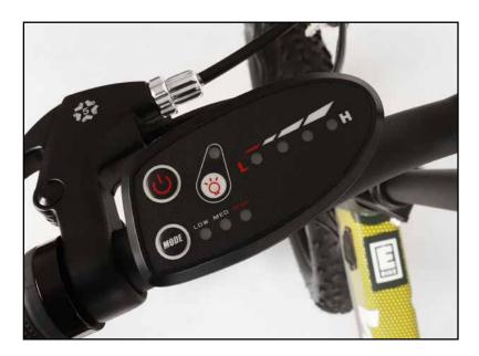
The power button is used to turn the motor on/off. To switch on, press once and to turn off, hold down the power button.
